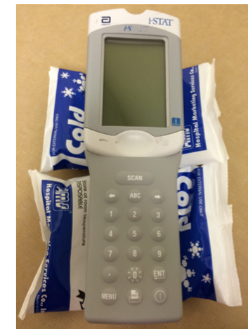
Figure 2. The device cradled in 2 chemical cold packs. During our event, we used a single larger cold pack.
